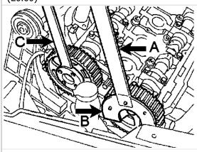
Loosen the camshaft gearwheel (inlet)
