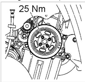
Remove the ancillary drive belt idler pulley (10.00)
