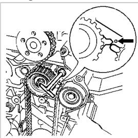
Tighten the tensioner pulley (25 Nm)
