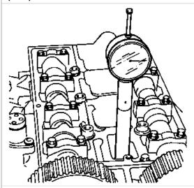
Turn the camshaft to TDC for cylinder  ${\bf 1}$
