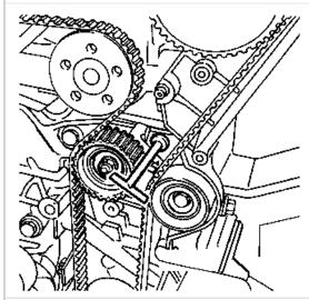
Tighten the tensioner pulley (25 Nm)
