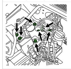
Remove the reinforcement plate on the lower cross member
